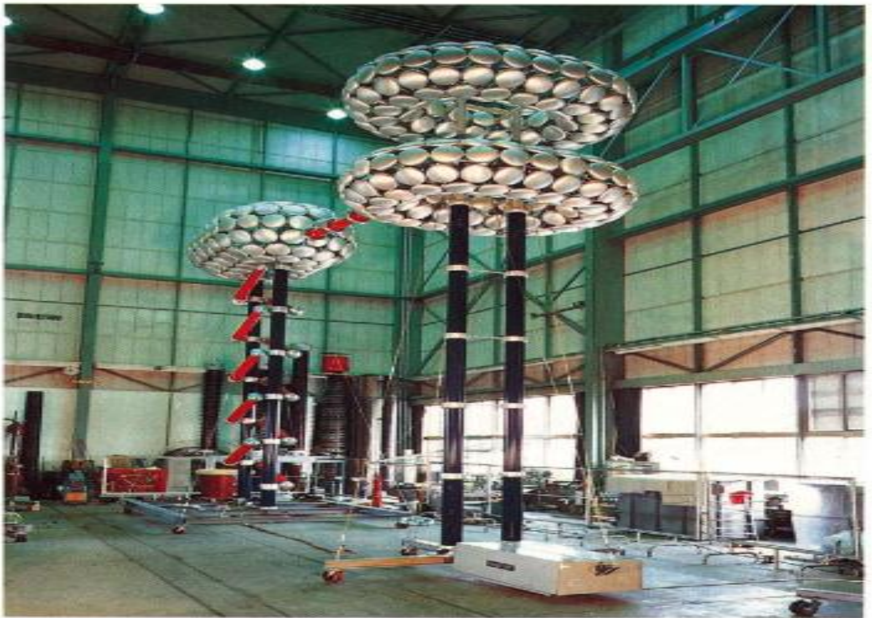
DC voltage test set 2000 kV, 10 mA for testing power cables, including a HV measuring resistor and automatic grounding system (foreground)
